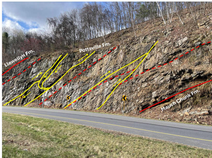
Figure 5.5. The Luzerne Outcrop showing formation contacts (red solid lines), bedding (red dashed lines), and some of the major faults (yellow solid lines).
