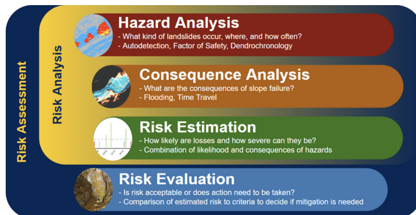
Figure 4.4. Overview of landslide risk assessment. Adapted from Macciotta et al. (2015). Included in this image are research contributions towards the overall risk assessment.
